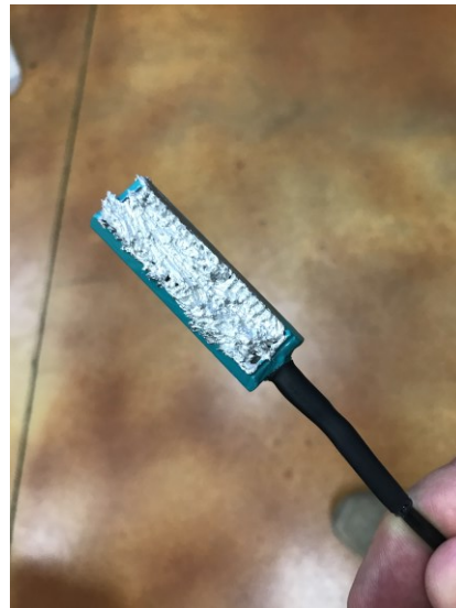
Figure 2- Attached with Conductive Epoxy
