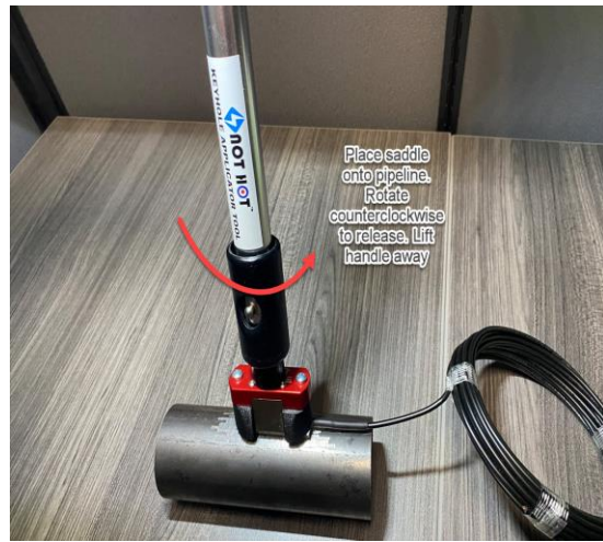
Figure 6- Applying Saddle on the Pipe
