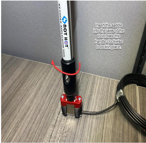
Figure 5- Saddle set into the Keyhole Tool
